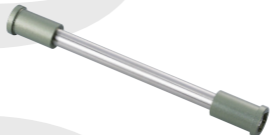
Hollow Chromoly Front Axle Shaft φ17(for JB/KYB φ41 Front Fork, incl. Nut) ¥19,000.-
