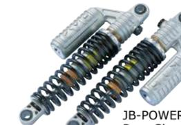
JB-POWER Rear Shock Absorber [Total Length 355mm] Kawasaki Type ¥ 75,000.- Spring Coil [increased Stiffness] ¥ 18,000.- Hook Wrench ¥ 3,000.-
